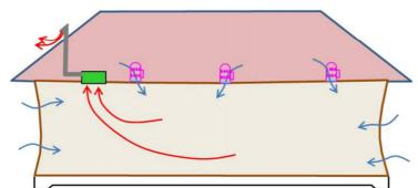
Figure 3 - With exhaust-only ventilation, the building is under negative pressure.
